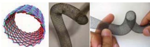
FIGURE 1. Left panel: synthetic picture of the multilayer stent. The middle panel, depicting the peripheral stent, and the right panel, depicting the aortic stent, show that whatever the tortuosity, the diameter of the stent remains unchanged, for the interlocked/ braided layers resist to distortion.
